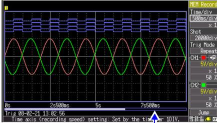
The portion of a waveform that is currently displayed can be confirmed by the position of the scroll bar.
