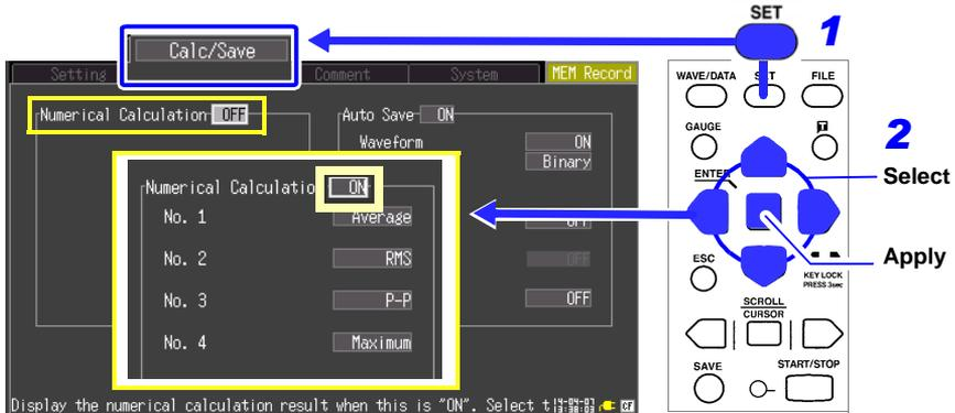
Set **Numerical Calculation** to **ON**, and select up to four calculation types for No. 1 through No. 4.
